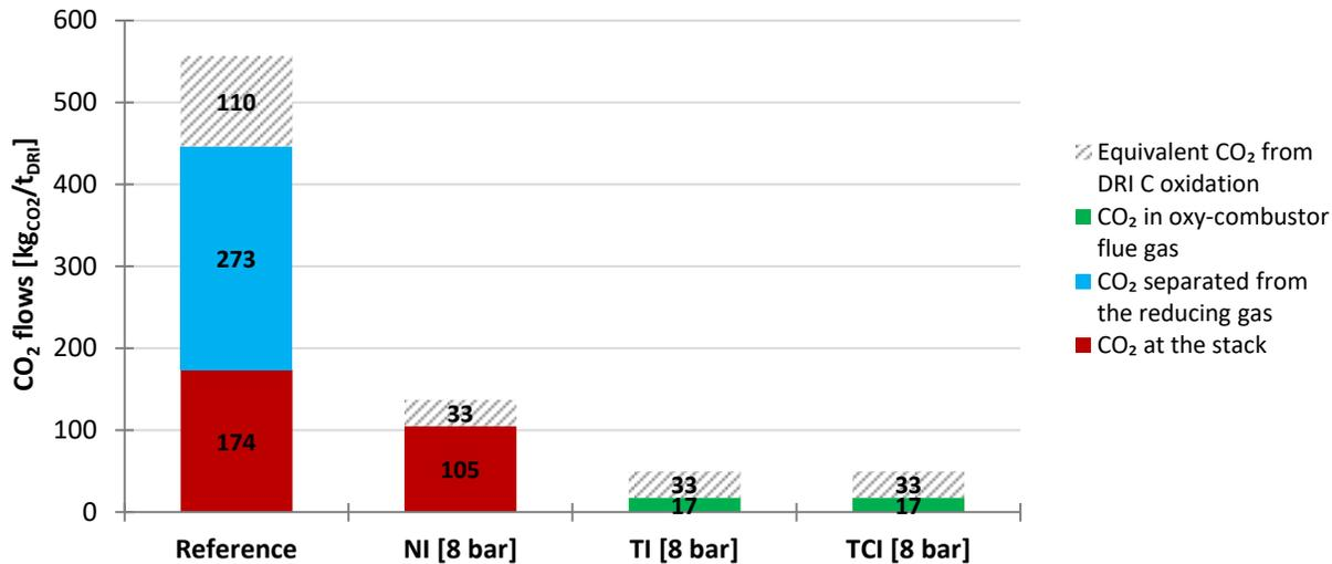
Energy and CO<sub>2</sub> balances of the reference case and three proposed configurations with a SOEC operating pressure of 8 bar
